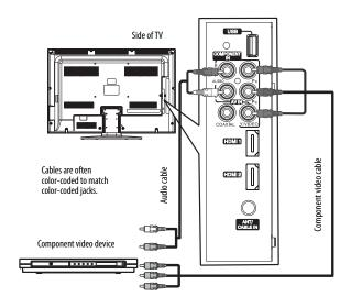
3 Connect an audio cable (not provided) to the L and R audio jacks on the side of your TV and to the L/R AUDIO OUT jacks on the component video device.
